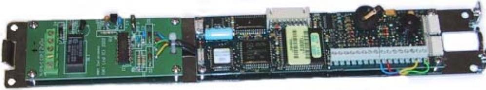
Mini-DCU shown with security cover removed
