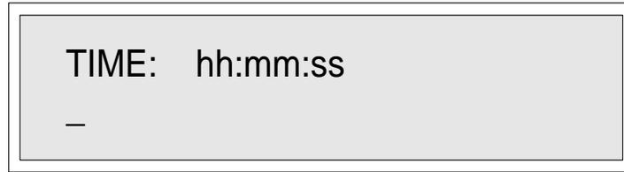
Enter the hours, minutes, and seconds in the format indicated and press **EXE**. This will cause the *Initial Options Menu* to appear (if this is the first use of the RAK and a password has not been established). If you have already established a password, the screen asking for entry of the password will appear.
