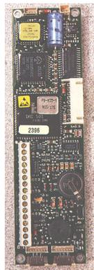
electronic controller has a built-in clock and calendar, allowing it to control access by time as well as location. This provides features such as time zones, holidays, and expiration dates. The controller automatically adjusts its clock for leap years and for daylight savings time. The controller's memory also retains an audit trail of the keys that have been used in it. There are controller housings available to fit any mounting arrangement.
